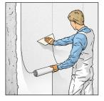
Place the wallcovering into the adhesive and press down with a wallpapering palette knife so that the adhesive is evenly distributed and a flat base surface is achieved.
