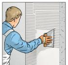
Use a toothed trowel (either C3 or B2 depending on the base surface) to evenly apply ERFURT-System Adhesive SR 4 perpendicular to the lengths of paper. To avoid adhesion problems, do not apply the adhesive too thinly and do not coat too large an area at once.
