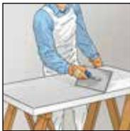
4. Use a toothed trowel/toothed comb to comb adhesive onto the insulating wedge (min. 8 mm tothing).
