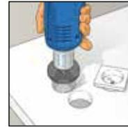
3. Use a keyhole saw to cut openings for sockets before fitting the panels.
