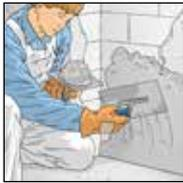
1. Fill cracks, chipped surfaces and seriously uneven surfaces with System Adhesive SR 6.
