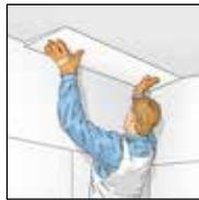
5. Press the insulating wedges onto the wall beside each other with moderate pressure. Remove excess adhesive along the edges.
