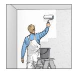
Using a long-pile roller, generously apply ERFURT-System Adhesive SR 2 evenly to the base surface over an area measuring the width of 1 or 2 strips.
